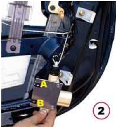
2) Photo 2 shows the motor assembly and its connecting rod in front of the right-side door at the position that it mounts to inside the door.
